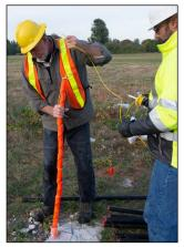
The ground vibrated for 29 seconds, almost enough time for observers to transition from a state of wonder to a state of concern. Students from Oregon State University and experts from Wallace Technical Blasting were experiencing a false earthquake, created by the detonation of multiple charges in 30- and 80-foot deep holes and designed to test how the surrounding soil would react.
