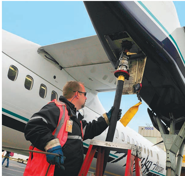
A member of the ground crew refuels one of Alaska's Bombardier Q400 aircraft.
