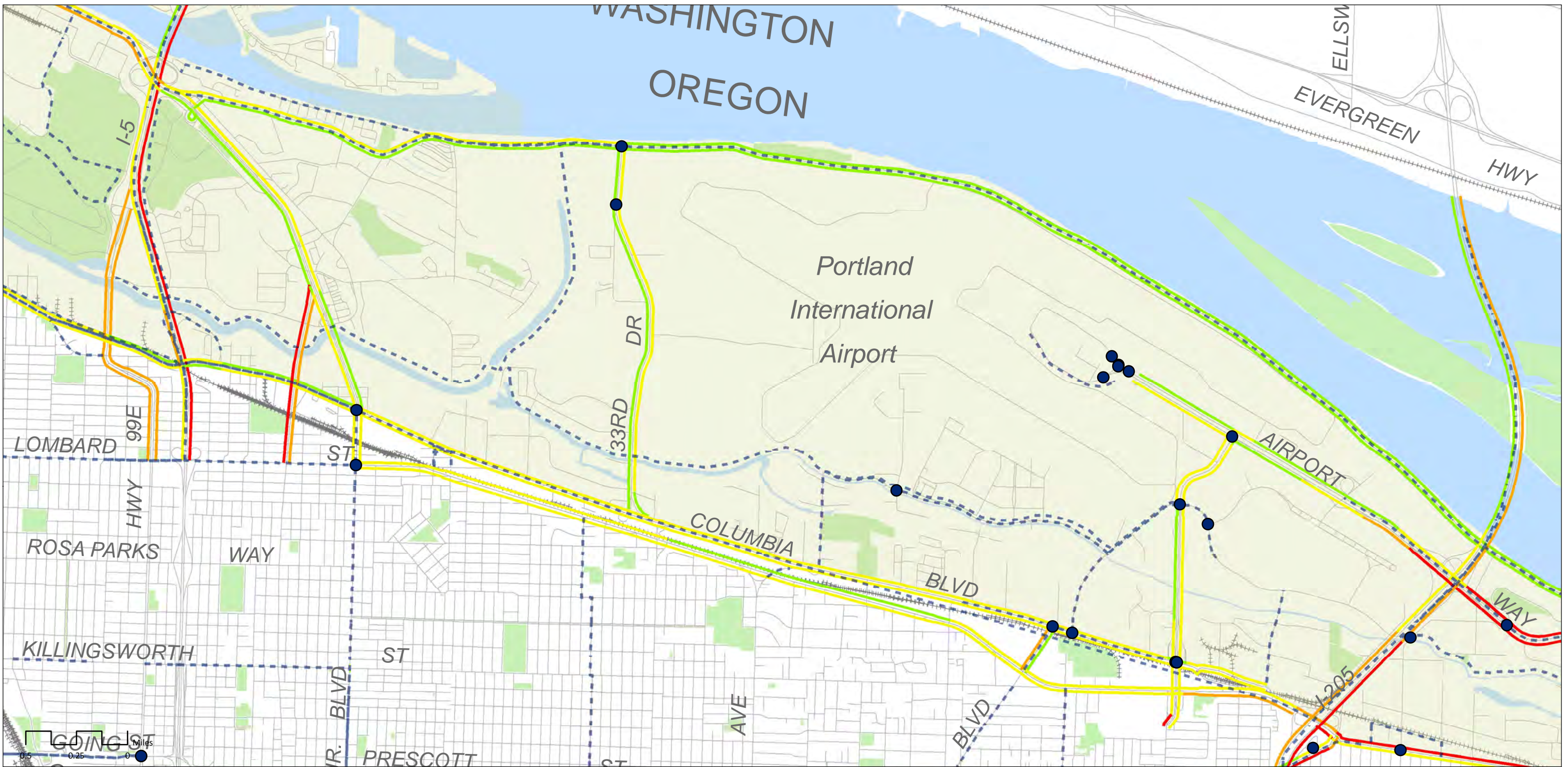
Figure 3b: Speed Map- 2008 to 2010 Weekday Evening Peak Hour (5-6 P.M.) Average Roadway Link Travel Speed compared to Free-Flow Speed
